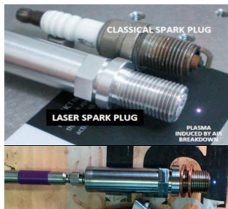
Figure. 3. A photo of a LASER spark plug is shown in comparison with a classical spark plug.
